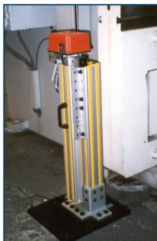
The laser assembly at bottom position.
