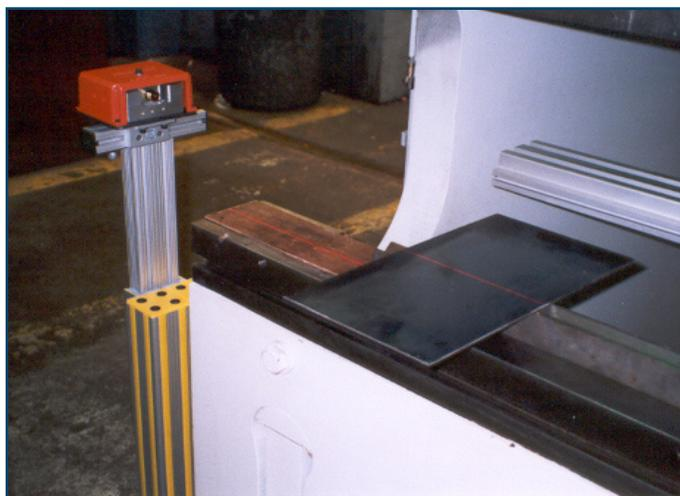
The laser unit projects a sharp, consistent line that may also be utilized on tandem press brakes.
